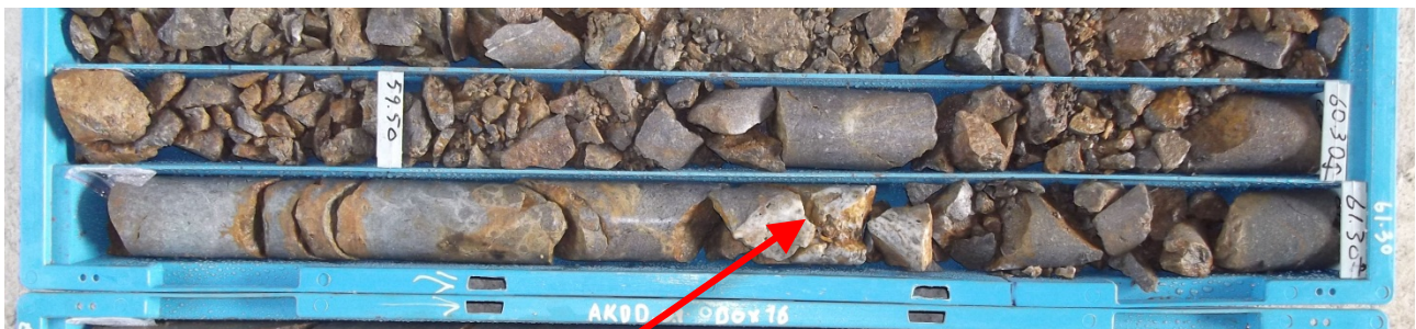
Quartz clasts showing multi depositional banding (vein?) with pervasively altered andesite clast in a hydrothermal breccia.
