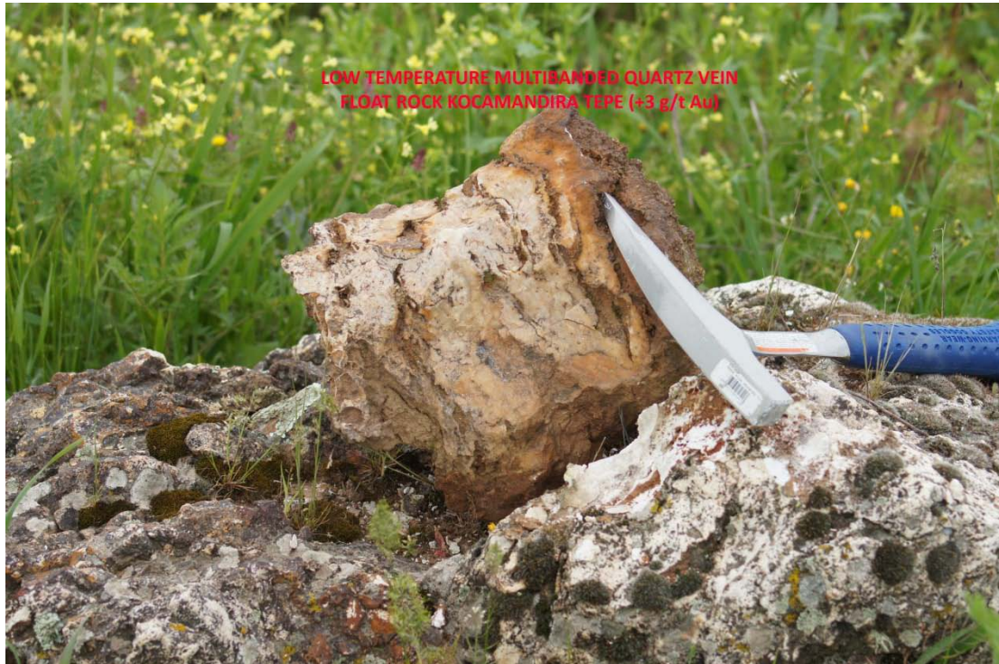
Figure 3 – Typical quartz vein found at Aktarma – note the typical low-sulphidation epithermal textures.
